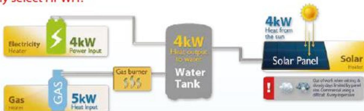
Comparison of the power needed to heat 1 ton water from 15°C to 55°C
