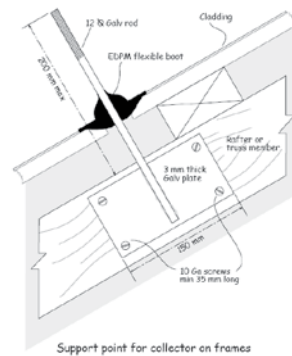
Figure 4: Panel stud fixing
